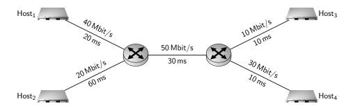
Figure 5.1: The maximum transmission rate and propagation delay is noted for each link.
