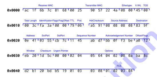
Figure 6.1: Hexdump of a complete Ethernet frame including FCS
