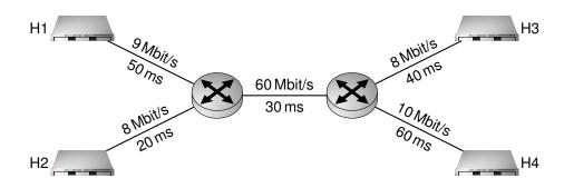
Figure 2.2: The latency and capacity is given for each link in the network.
