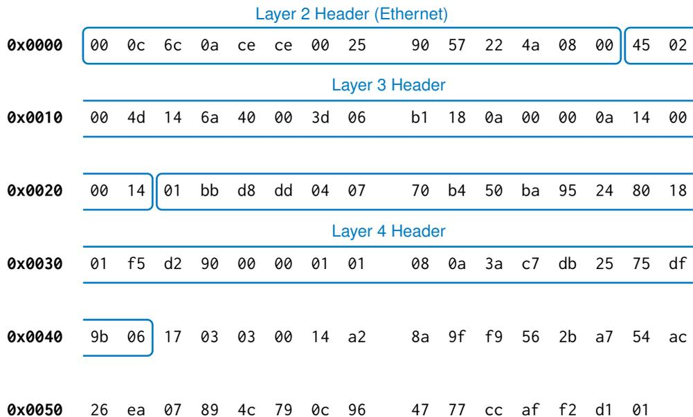
Figure 5.1: Hexdump of an Ethernet frame including FCS
