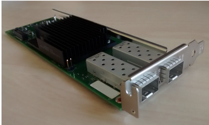
Figure 9: NIC with two slots for pluggable transceivers
