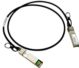
Figure 11: Direct-Attach Copper (DAC) twinaxial cable with integrated SFP modules (cheap, used for low range connections \leq 15 m)
